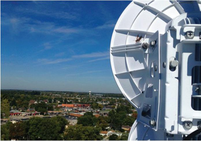
Wireless Internet service providers (WISPs) use tower-mounted antennas to transmit and receive radio signals, much as cellular service providers do.
